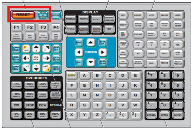
Figure 4. Haas CNC Mill controls with “Reset” and “Power Up/Restart” hard keys outlined in red
